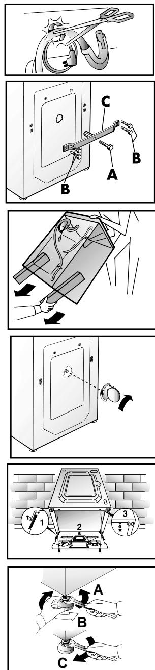
Note: we recommend you keep the transverse bracket, braces and screws to immobilise the machine for future transit. The Manufacturers will not be responsible for any possible damage to the machine caused by not following the rules relating to releasing the mechanism. The user is responsible for all costs of installation.
